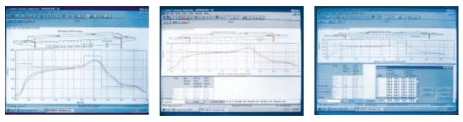
Figure 1. Thermal profiling software records events taking place during the thermal process and displays them for immediate viewing or stores them for later recall and analysis.
